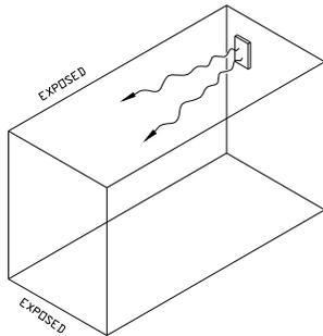
Where one or two walls are exposed to outside environment in smaller building areas, a single unit placed like this may be sufficient.
