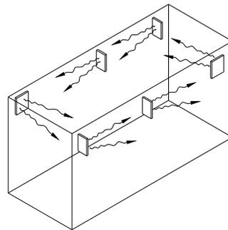
Larger building areas may require multiple units installed like this, especially where three or more walls are exposed to outside environment. Units should be arranged for providing perimeter air circulation where the air stream of one supports that of another.
