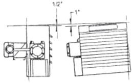
Maximum tilt allowed during operation (applicable front to back and side to side in either direction). Heater must be permanently mounted.
